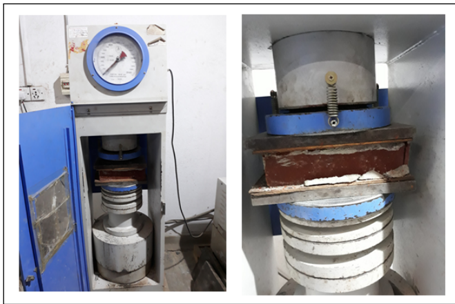
Figure 4: Compressive strength testing
