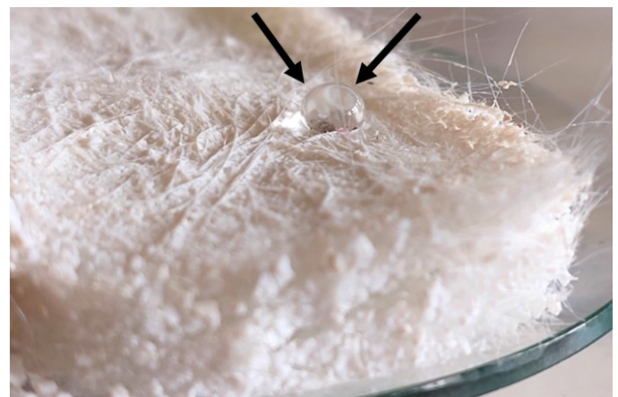
Figure 21: Visual inspection of WW2 for hydrophobicity after heating at 200°C
