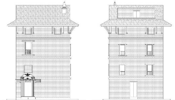
Figure 6: North and south elevations of Lakhe Chhen after reconstruction
