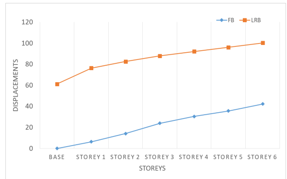
Figure 17: Lateral Displacement of 6 storey building in X direction
