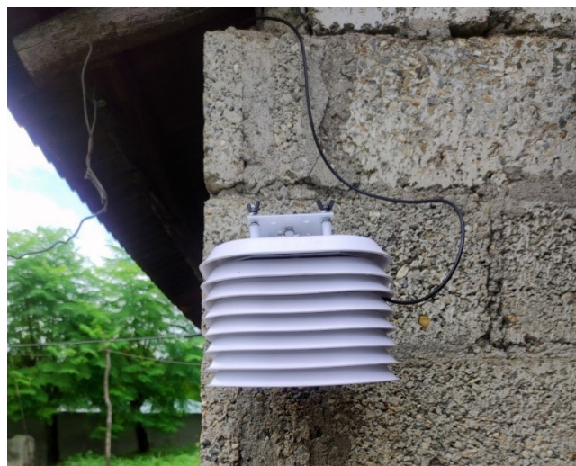
Figure 2: Outdoor Sensor with Solar Radiation Shield
