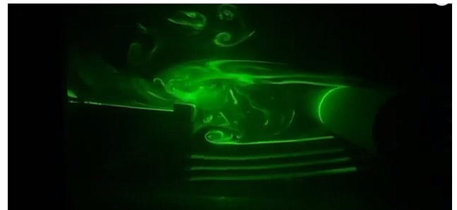
Figure 15: Flow Visualization at Re = 1354 at wind tunnel in Pulchowk Campus.
