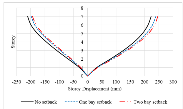
Figure 12: Maximum Storey Displacement of 7-storey building (3-7 case)
