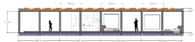
Figure 6: Section of the module
