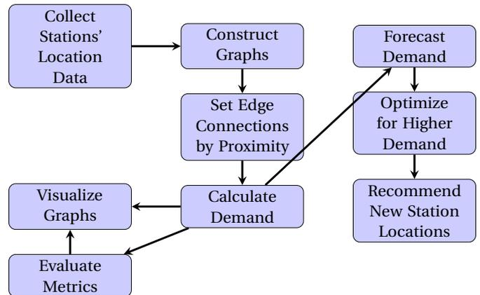
Figure 5: Block Diagram for Charging Station Data Analysis and Optimization
