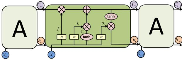
Figure 4: Structure of LSTM
