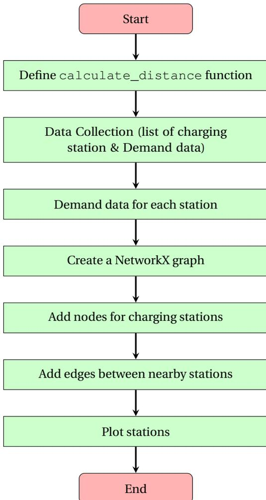
**Figure 6:** Flowchart for the Graph construction(GNN)
