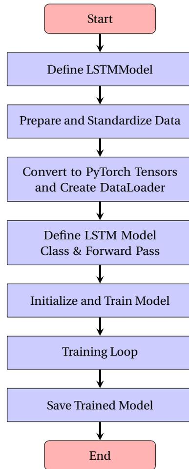
**Figure 7:** Flowchart for LSTM Model (Load Forecasting)
