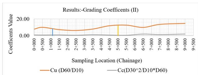
Figure 11: Grading coefficient of sediment
