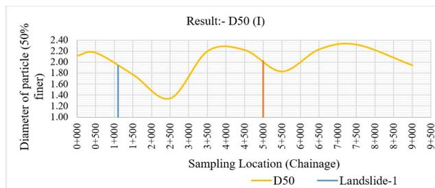
Figure 12: Mean size particle of sediment.
