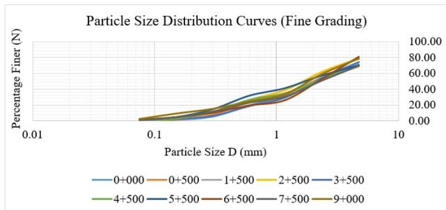
Figure 8: Particel size distribution curve (Fine Grading)
