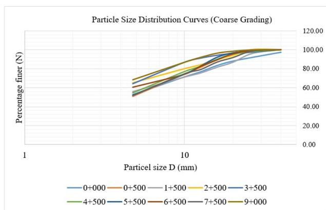
Figure 9: Particle size distribution curve (Coarse Grading).
