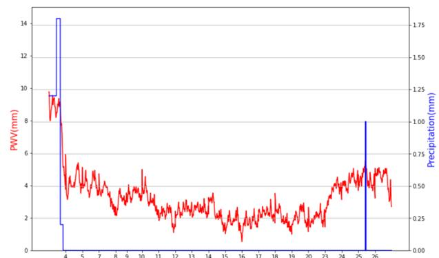
**Figure 9:** Precipitable water vapor versus precipitation during (December-2021, Nagarkot GNSS station).
