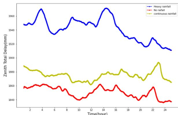
Figure 2: Comparison of Zenith Total delay at Nagarkot GNSS Station
