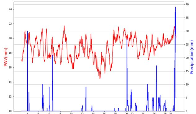
**Figure 7:** Precipitable water vapor versus Precipitation (July-2022, Pokhara GNSS station)
