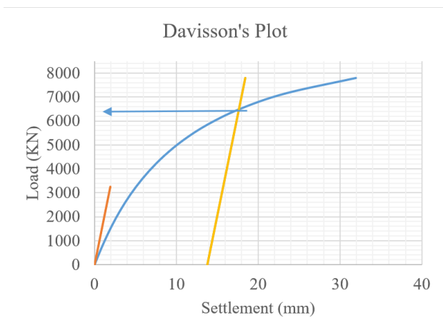
Figure 8: Davisson's Plot for Left Abutment Pile
