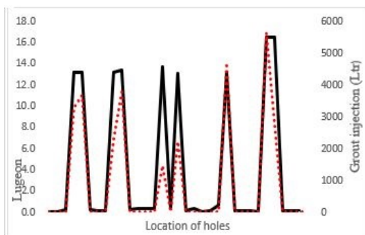
Figure 4: Lugeon Vs grout volume for packer setting at 5m @Bhaise adit gate
