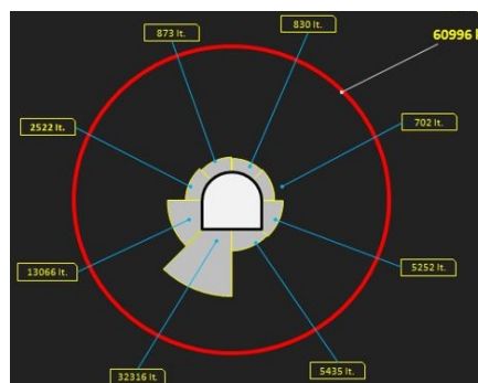
Figure 8: Comparison of volume of grout injection around tunnel profile at HT1 looking D/S
