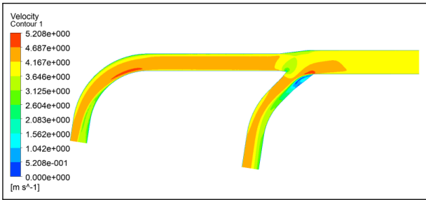
Figure 11: Velocity distribution at mid-plane
