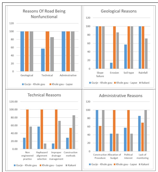
Figure 5: Reason for road to be inoperative
