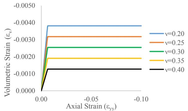
**Figure 12:** Relation between volumetric and axial strain obtained from triaxial test simulation for varying Poisson's ratio
