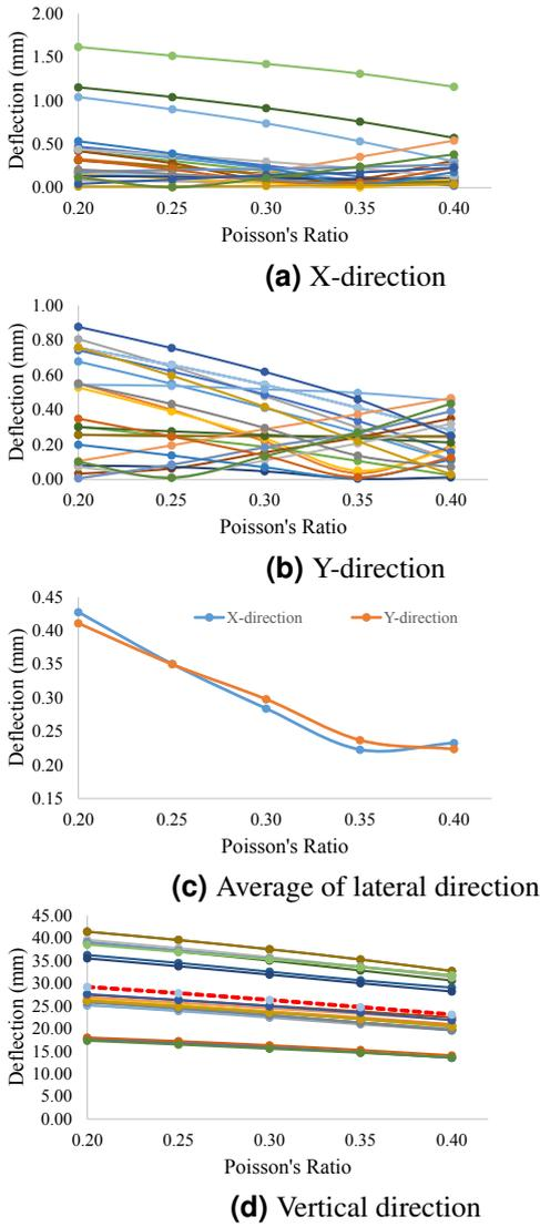
**Figure 9:** Absolute deformation of soil with varying Poisson's ratio
