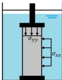
**Figure 10:** Triaxial test simulation model
