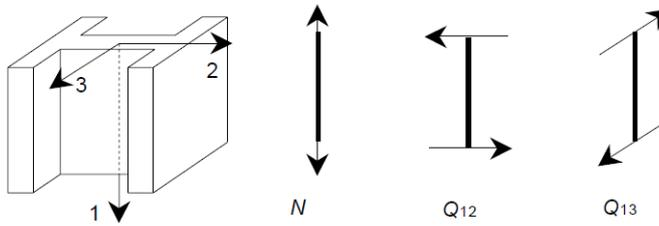
Figure 6: Shear and axial forces
