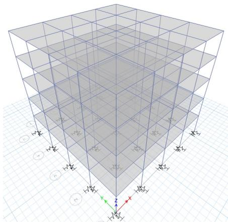
Figure 7: 3D structural modelling with spring support
