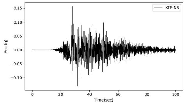
Figure 3: Strong motion seismogram recorded at Kirtipur during Gorkha earthquake
