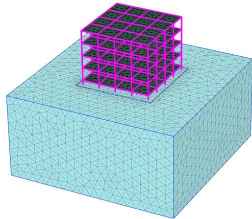
Figure 5: Generated mesh for finite element analysis
