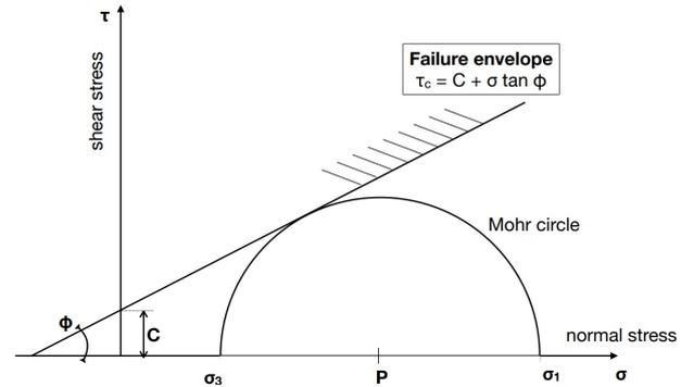
**Figure 2:** The MC failure criteria and Mohr's circle [4]
