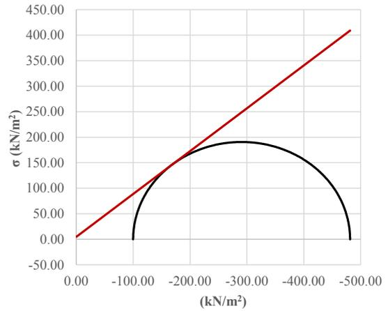
**Figure 11:** Mohr-Coulomb circle and failure envelope obtained from simulation
