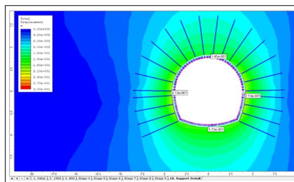
**Figure 10:** Deformation after Installation of Support
