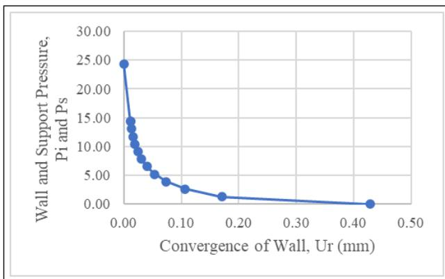
**Figure 5:** Ground Reaction Curve (GRC)
