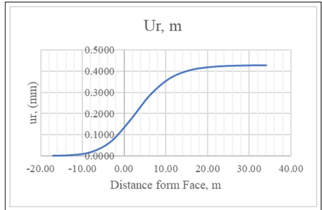
**Figure 6:** Longitudinal Displacement Profile (LDP)
