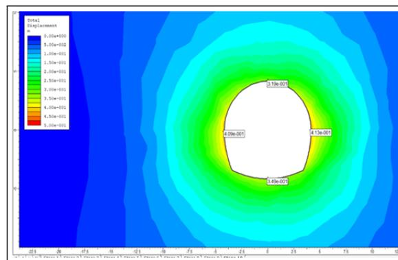
**Figure 9:** Deformation before installation of support and Plastic zone Radius
