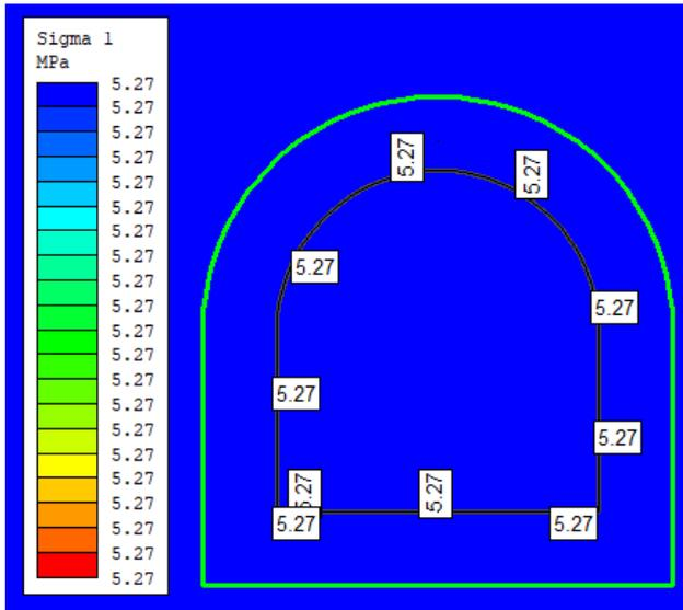
Figure 9: Tunnel section used in Phase 2 (4.3\*4.6)
