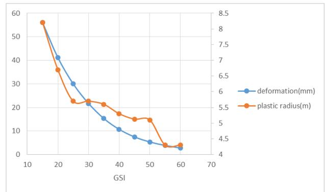
Figure 12: Variation of deformation and plastic radius with respect to GSI
