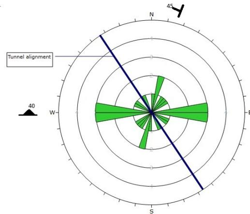
**Figure 8:** Tunnel alignment based on joint orientation
