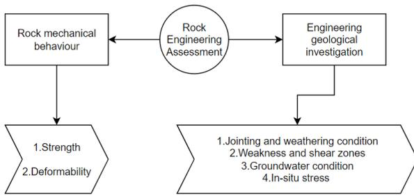
Figure 1: Parameters for rock engineering assessment
