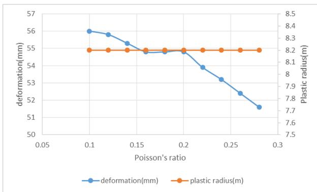
Figure 10: Variation of deformation and plastic radius with respect to poisson’s ratio
