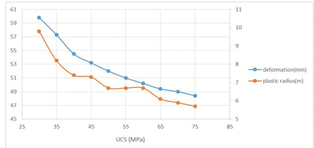
Figure 11: Variation of deformation and plastic radius with respect to UCS
