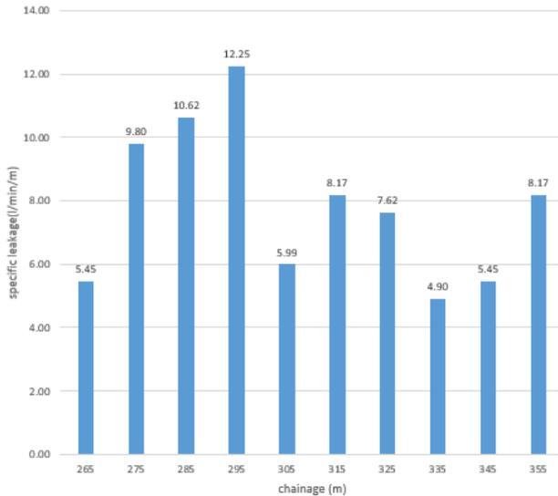
**Figure 7:** Leakage estimation in unlined headrace tunnel
