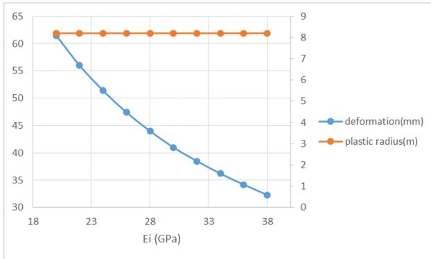
**Figure 13:** Variation of deformation and plastic radius with respect to  $E_i$
