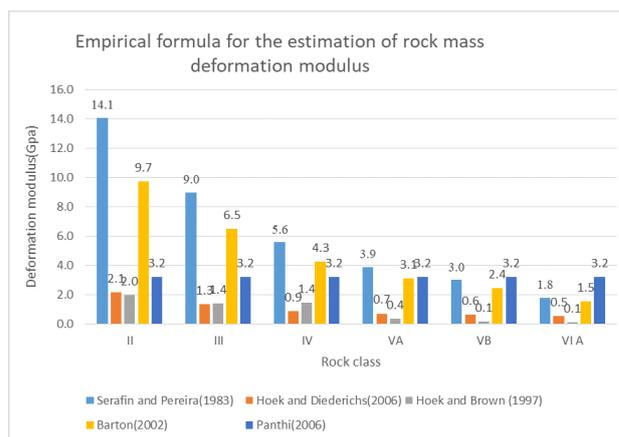
Figure 6: Comparison of deformation modulus using different empirical methods
