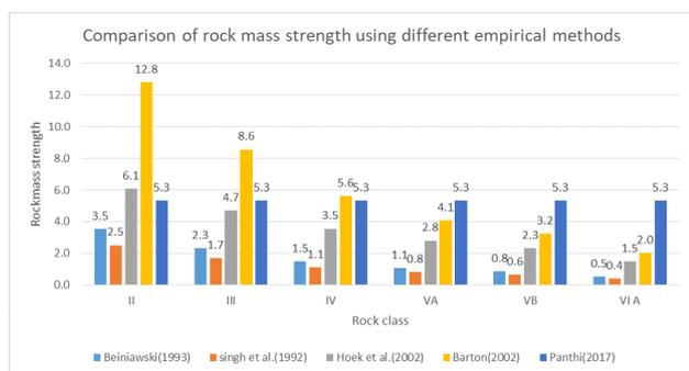
Figure 5: Comparison of rock mass strength using different empirical methods
