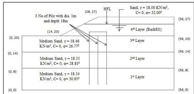
Figure 4: Sample Model of Katnu Khola River Bridge Abutment-1
