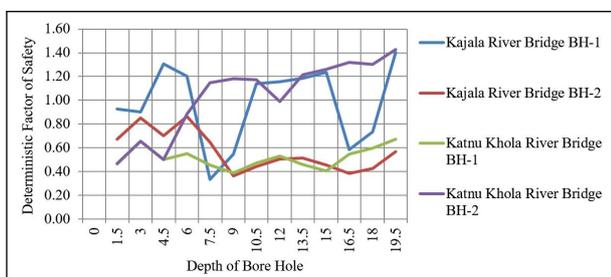
**Figure 5:** Deterministic Factor of Safety VS Depth of Bore Hole
