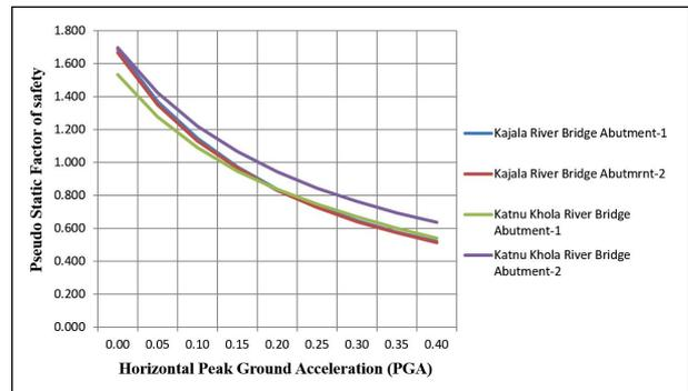
**Figure 6:** Pseudo Static Factor of Safety VS PGA at Zero Horizontal Pile Load
