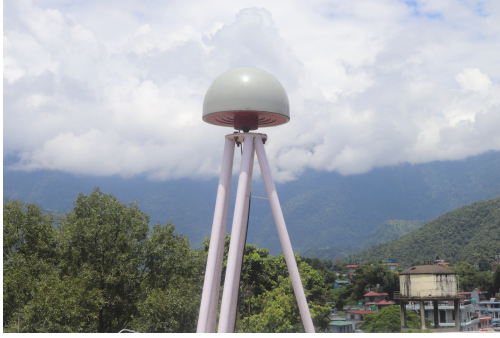
Figure 7: GNSS receiver’s antenna
