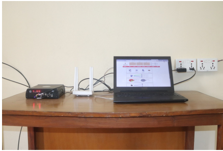
Figure 8: GNSS receiver data logging and processing setup
