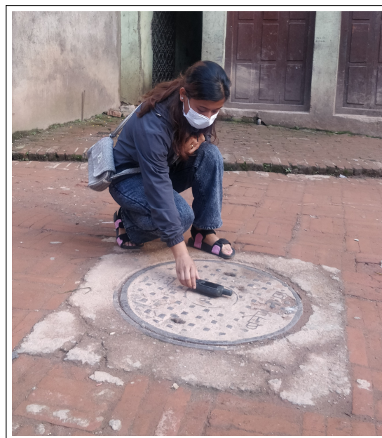
Figure 6: Site Survey for Nodes surface elevation
