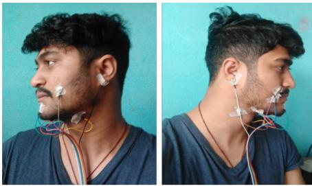
Figure 2: OpenBCI Electrodes Placement
