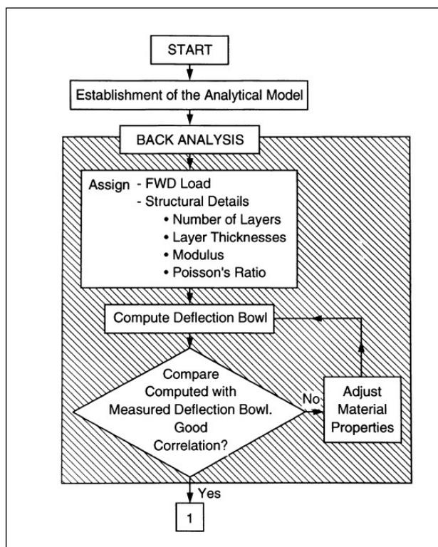
Figure 1: Typical Back Calculation Process
