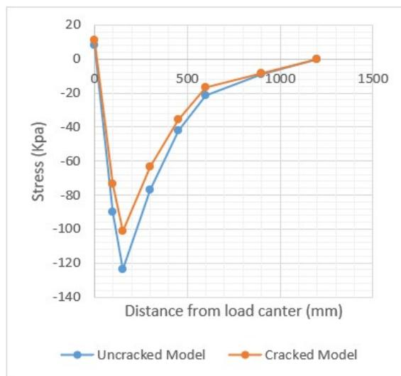
**Figure 10:** Shear stresses at the bottom of bituminous surface layer
