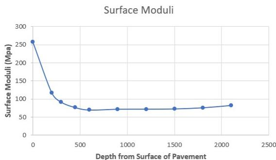
**Figure 4:** Variation of Surface Modulus along the depth
