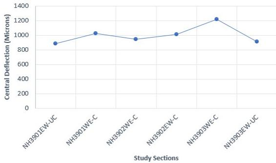
**Figure 3:** Normalized Center Deflection across the Pavement Sections
