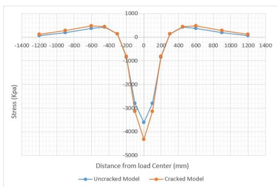
**Figure 7:** Horizontal stresses at the bottom of the bituminous surface layer
