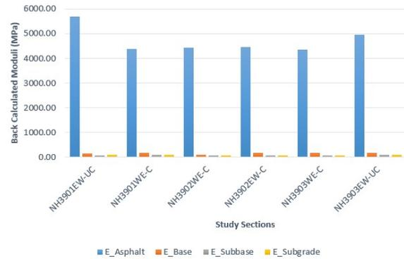
**Figure 5:** Average Back Calculated Moduli
