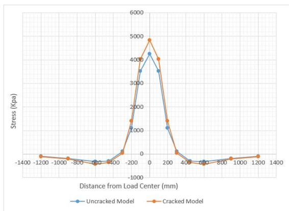
**Figure 6:** Horizontal stresses at the surface of the bituminous surface layer
