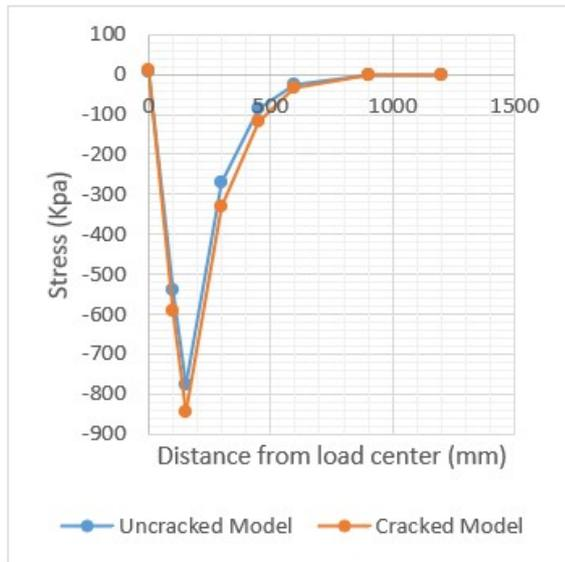
**Figure 9:** Shear stresses at the middle of bituminous surface layer
