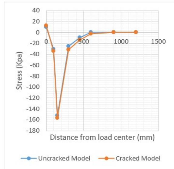
**Figure 8:** Shear stresses at the surface of bituminous surface layer
