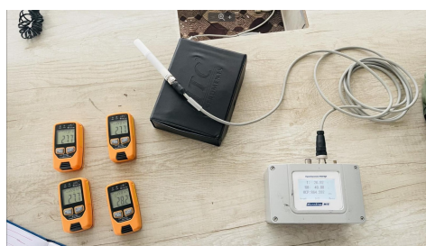
Figure 5: Calibration of Thermometers at DHM
