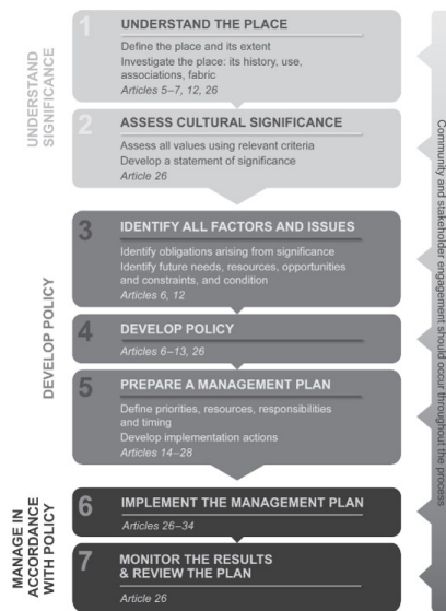
Figure 1: The Burra Charter Process of Architectural Conservation
