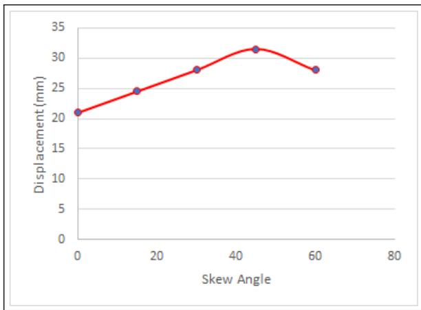
**Figure 11:** Pier top displacement for Slight Damage
