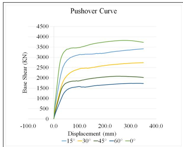
**Figure 10:** Pushover Curve for different skew angles
