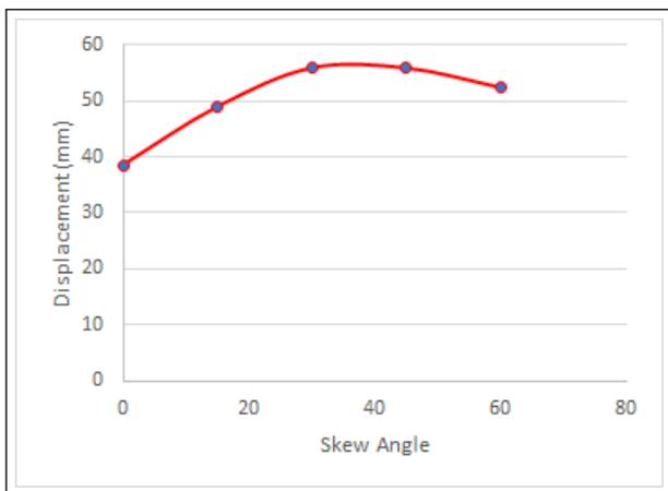
**Figure 12:** Pier top displacement for Moderate Damage
