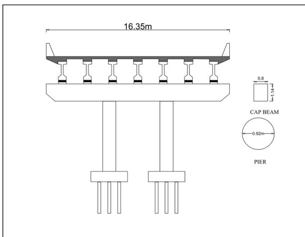
Figure 3: Cross Section of Bridge
