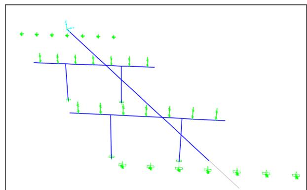
Figure 6: Beam stick FEM model for 30°
