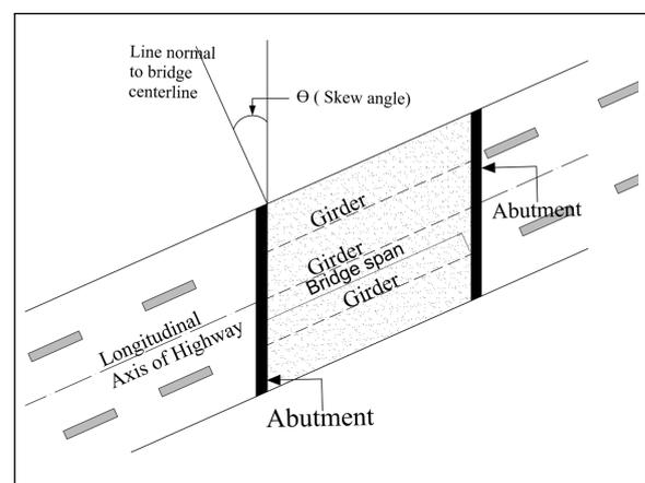
Figure 1: Plan of Skew Bridge
