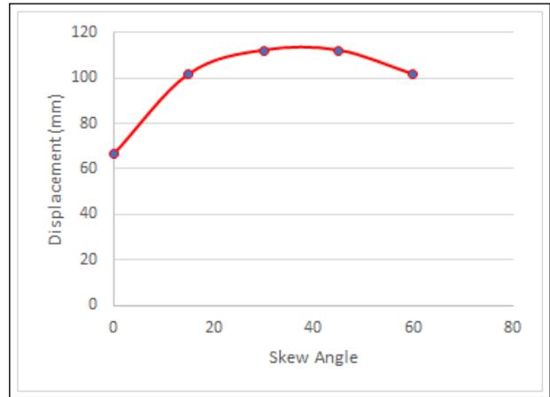
**Figure 13:** Pier top displacement for Extensive Damage
