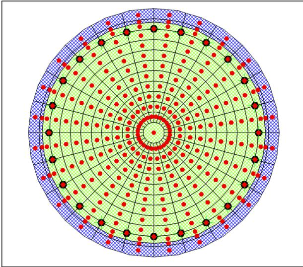
Figure 9: Fiber Layout of Pier Section
