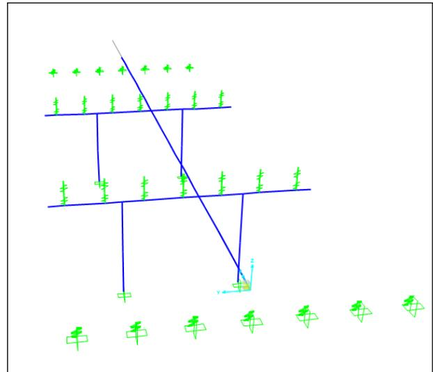
Figure 4: Beam stick FEM model for 0°
