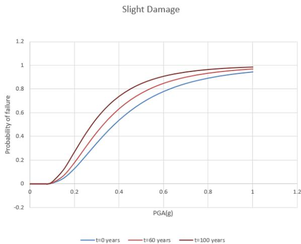
Figure 5: Fragility curve for Slight Damage at different time period
