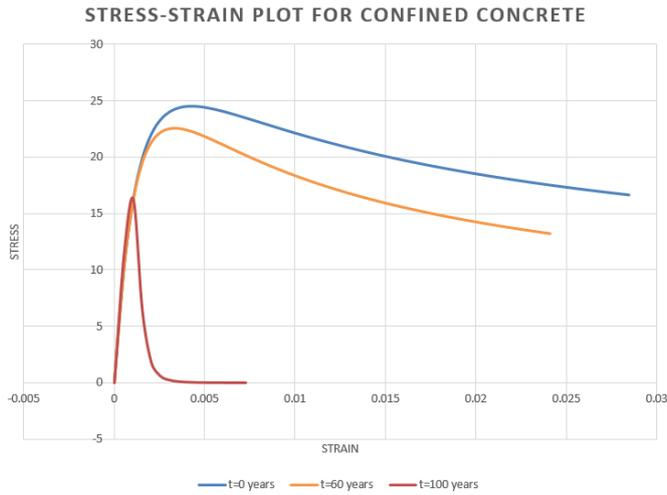
Figure 3: Stress-Strain plot for confined concrete at different time period
