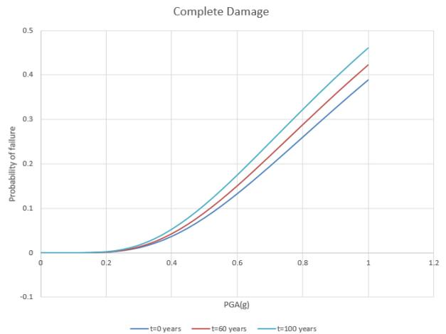
Figure 8: Fragility curve for Complete Damage at different time period
