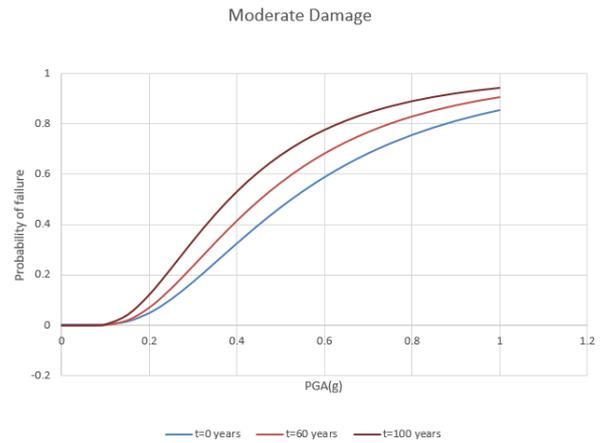
Figure 6: Fragility curve for Moderate Damage at different time period
