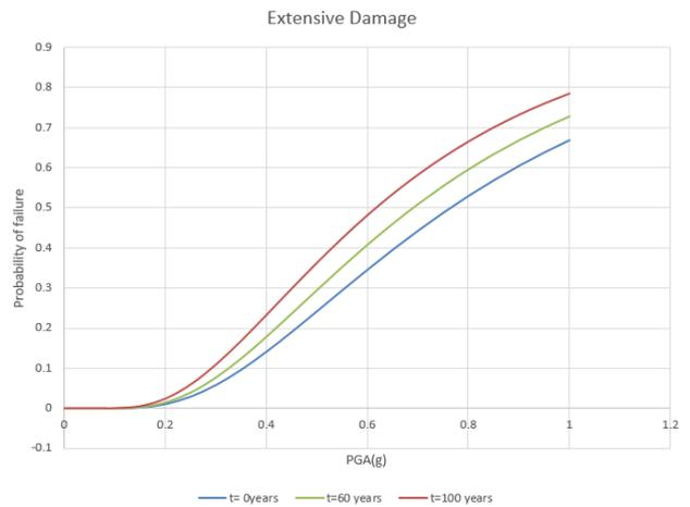
Figure 7: Fragility curve for Extensive Damage at different time period
