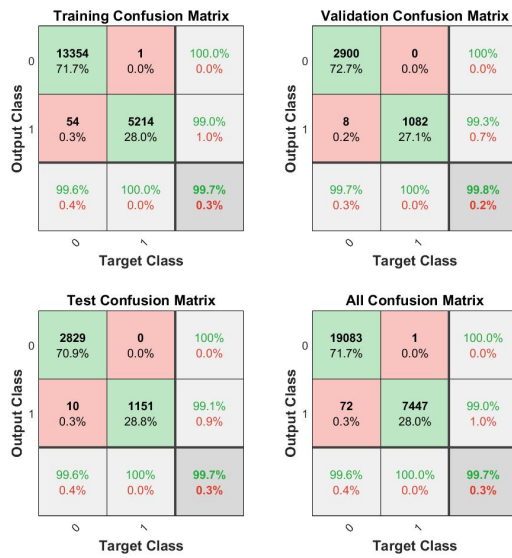
Figure 6: Confusion Matrix of Fault Classification in phase A
