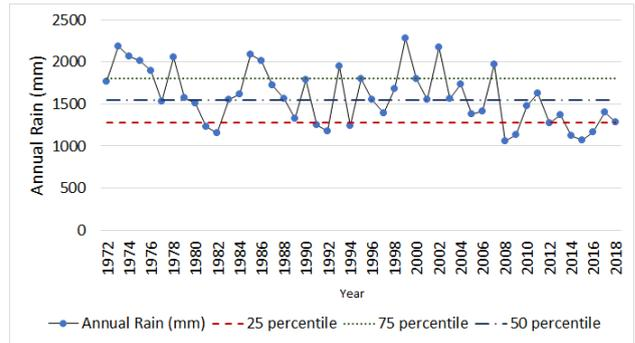
Figure 2: Annual rainfall showing 25 percentile, 50 percentile, and 75 percentile line to classify years in to dry, average, and wet years
