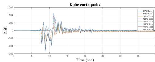
Figure 11: Drift vs time of the bridge due to Kobe earthquake at different scale factors
