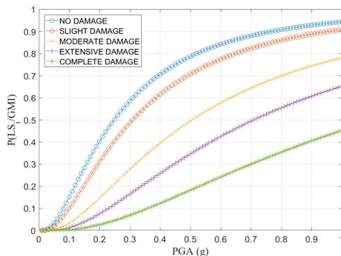
**Figure 13:** Fragility curves of pier of Bijaypur Bridge for various damage states
