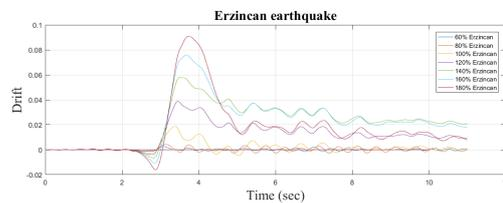
Figure 9: Drift vs time of the bridge due to Erzincan earthquake at different scale factors
