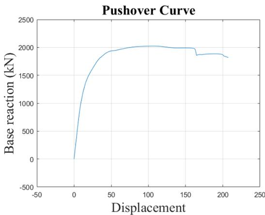
Figure 7: Pushover curve of the pier of the bridge
