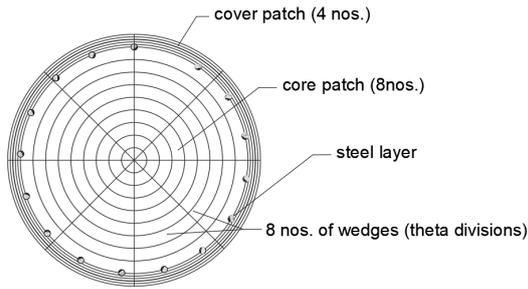
Figure 5: Fiber section of the pier
