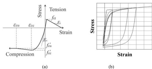
Figure 2: Adopted constitutive material models: (a) Concrete02, (b) Steel02 with isotropic hardening
