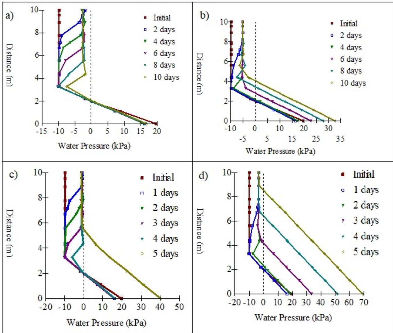
**Figure 5:** Relationship between porewater pressure at various depths and rainfall duration for a)  $I= 4 \text{ mm/h}$ ,  $k_s= 36 \text{ mm/h}$ ; b)  $I= 4 \text{ mm/h}$ ,  $k_s= 360 \text{ mm/h}$ ; c)  $I= 16 \text{ mm/h}$ ,  $k_s= 36 \text{ mm/h}$ ; d)  $I= 16 \text{ mm/h}$ ,  $k_s= 360 \text{ mm/h}$
