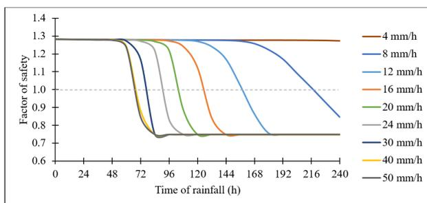
**Figure 7:** Factor of safety versus rainfall duration under various rainfall intensities for  $k_s = 36$  mm/h
