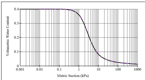
Figure 2: Volumetric water content function
