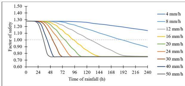
**Figure 6:** Factor of safety versus rainfall duration under different rainfall intensities for  $k_s = 360$  mm/h
