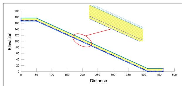
Figure 4: Geometrical model of slope and boundary condition used in numerical modelling
