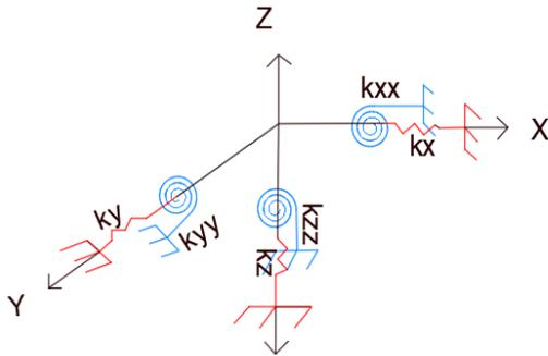
Figure 1: Equivalent spring model along 6 DOF
