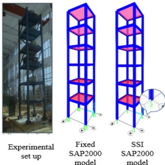
Figure 3: FEM modelling of experimental setup
