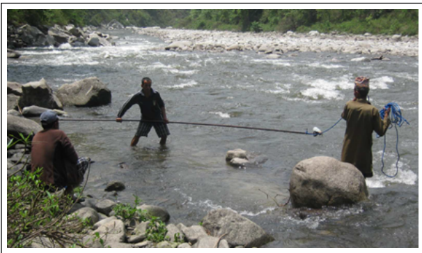
Figure 3: Suspended sediment sampling process in the field [12]
