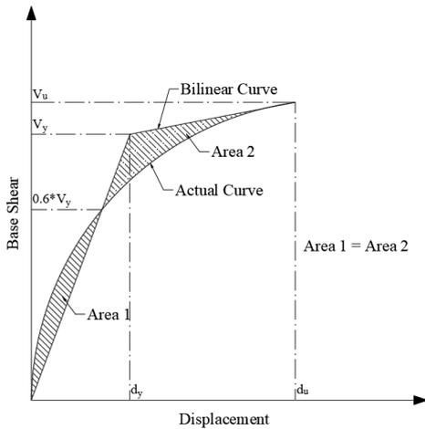
Figure 2: Bilinear Idealization of Pushover Curve
