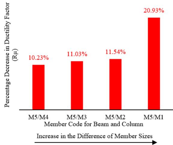
**Figure 10:** Effect on Ductility Factor by Difference in Member Sizes
