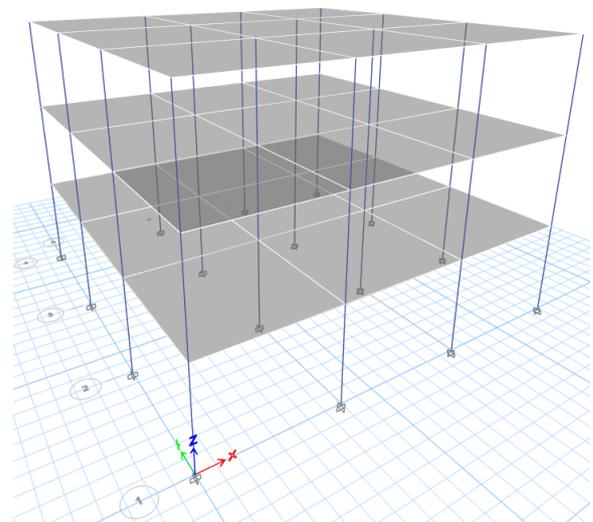
**Figure 1:** Finite Element Modelling of 3 Storey 3 Bay 4m Bay Length (3S3B4BLM2) Model
