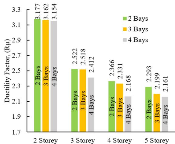
Figure 7: Ductility factor for number of bay for various number of storey
