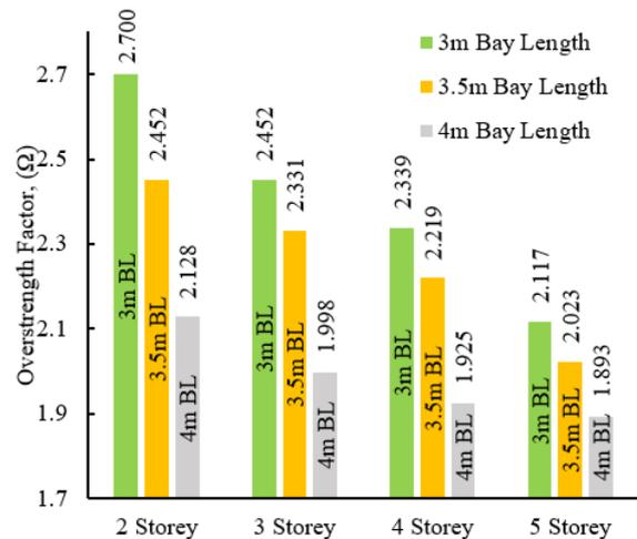
Figure 4: Overstrength factor for bay length for various number of storey
