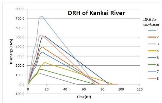
**Figure 3:** Direct Runoff Hydrograph of Sub Basin for 100yrs return period
