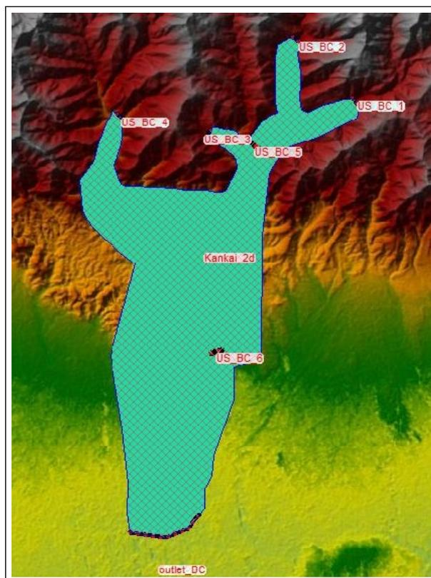
**Figure 4:** 2D mesh and Boundary Condition in Modelling
