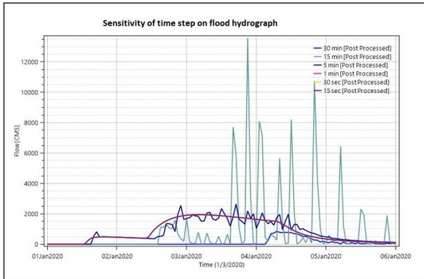
**Figure 7:** Sensitivity of time step on Flood Hydrograph
