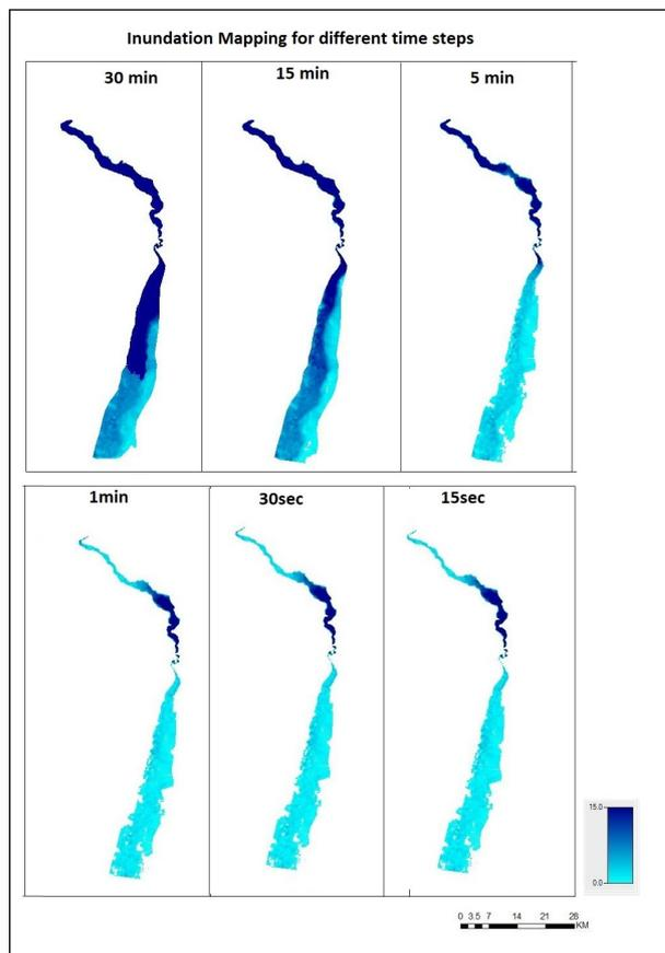
**Figure 6:** sensitivity of time step on Inundation Area
