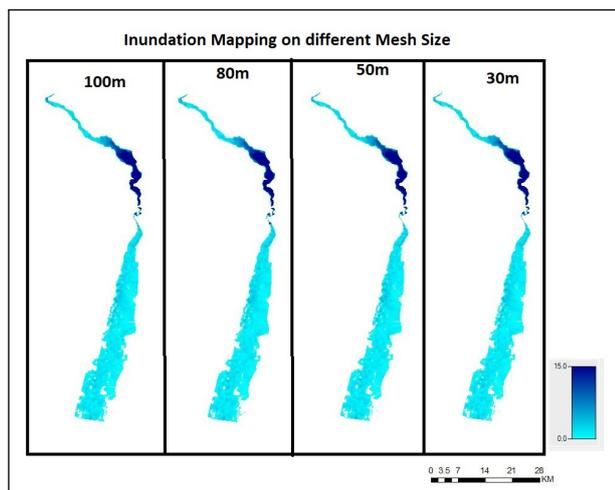
**Figure 5:** Inundation on different Mesh Geometry
