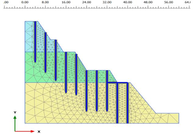
**Figure 9:** Slope model with hTP pile at bottom
