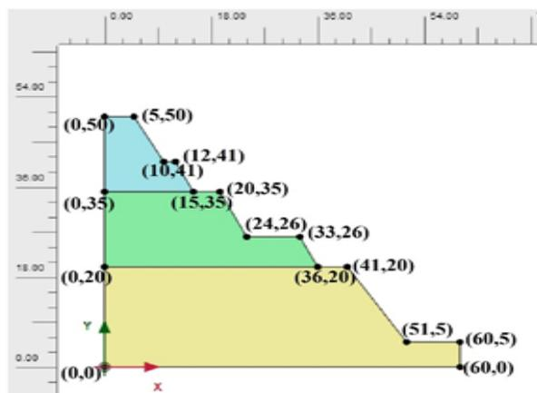
**Figure 5:** Geometric model of the slope
