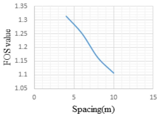
Figure 17: Factor of Safety vs Spacing of piles
