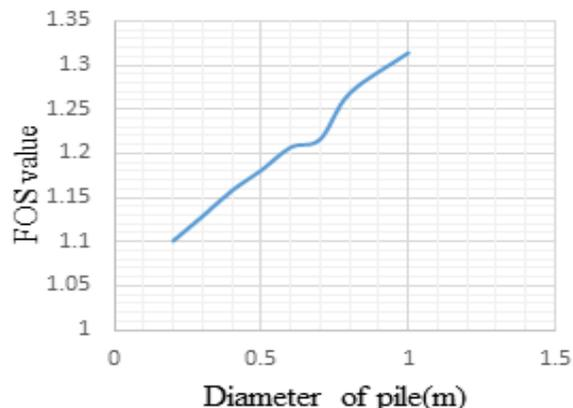
**Figure 15:** Factor of Safety vs Diameter of pile
