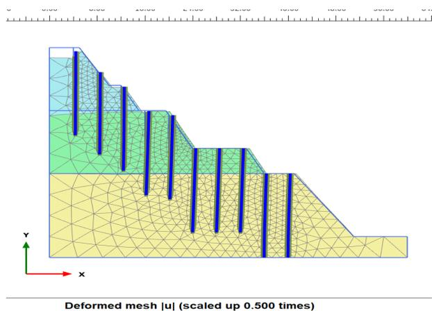
**Figure 14:** Deformed mesh of slope with vertical piles
