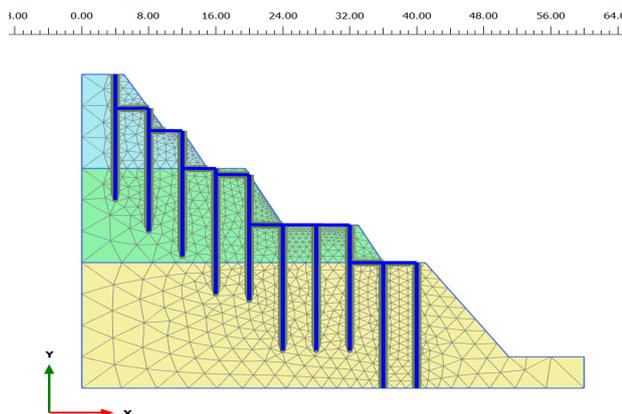
**Figure 13:** Slope model with hTP pile at every section
