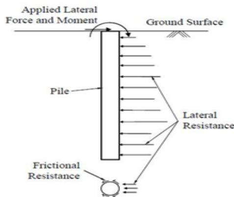
**Figure 3:** Mechanism of resisting lateral load by pile [3]
