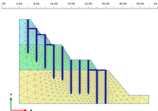
Figure 11: Slope model with hTP pile at top and bottom
