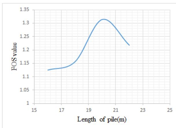
**Figure 16:** Factor of Safety vs Length of pile
