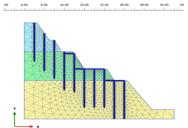
Figure 12: Slope model with hTP pile at middle and bottom
