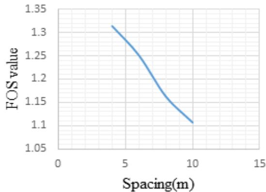
Figure 17: Factor of Safety vs Spacing of piles
