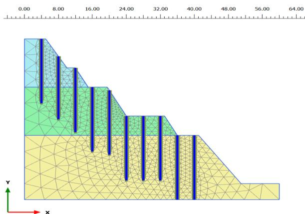
**Figure 6:** Slope Model with vertical pile
