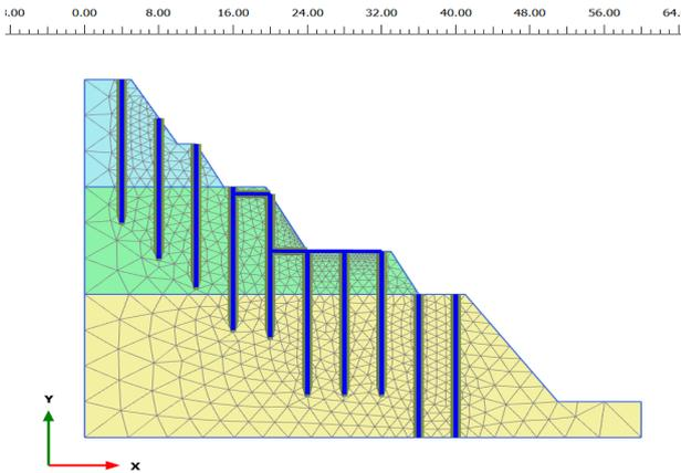
Figure 8: Slope model with hTP pile at middle
