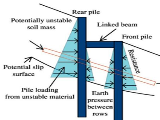
**Figure 4:** Mechanical model of hTP [4]
