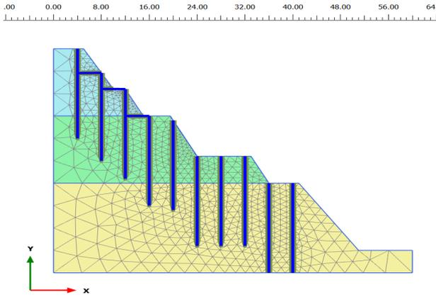
Figure 7: Slope model with hTP pile at top
