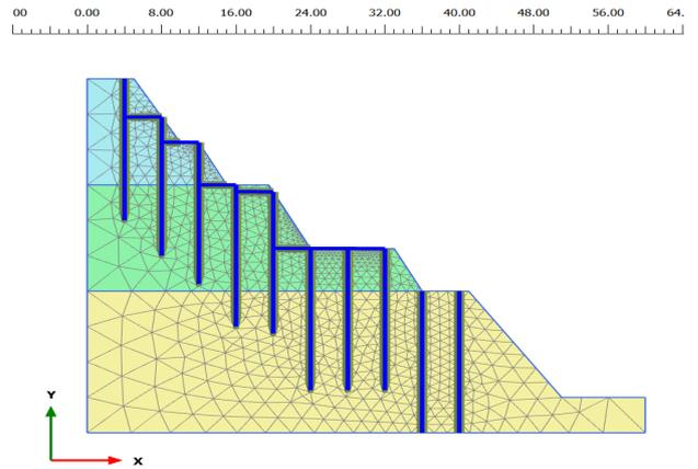
Figure 10: Slope model with hTP pile at top and middle
