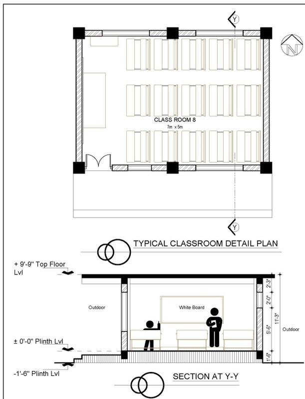
Figure 12: Detail floor plan and section of Shree Kankali Secondary School Classroom
