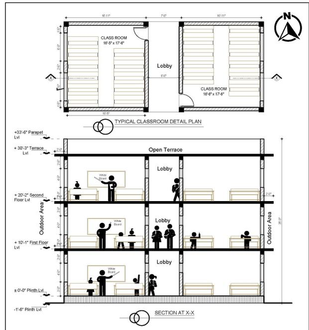
**Figure 10:** Typical Classrooms floor plan and Detail section of Gyanodaya Secondary School
