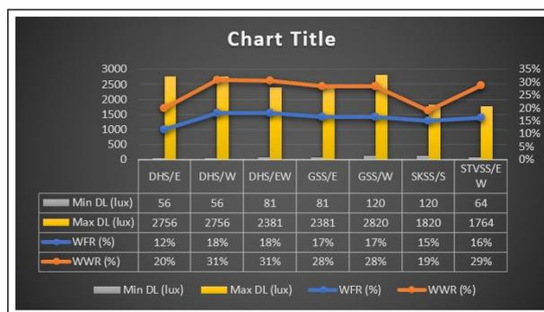
Figure 20: WWR, WFR and Daylight level comparison chart of case studies
