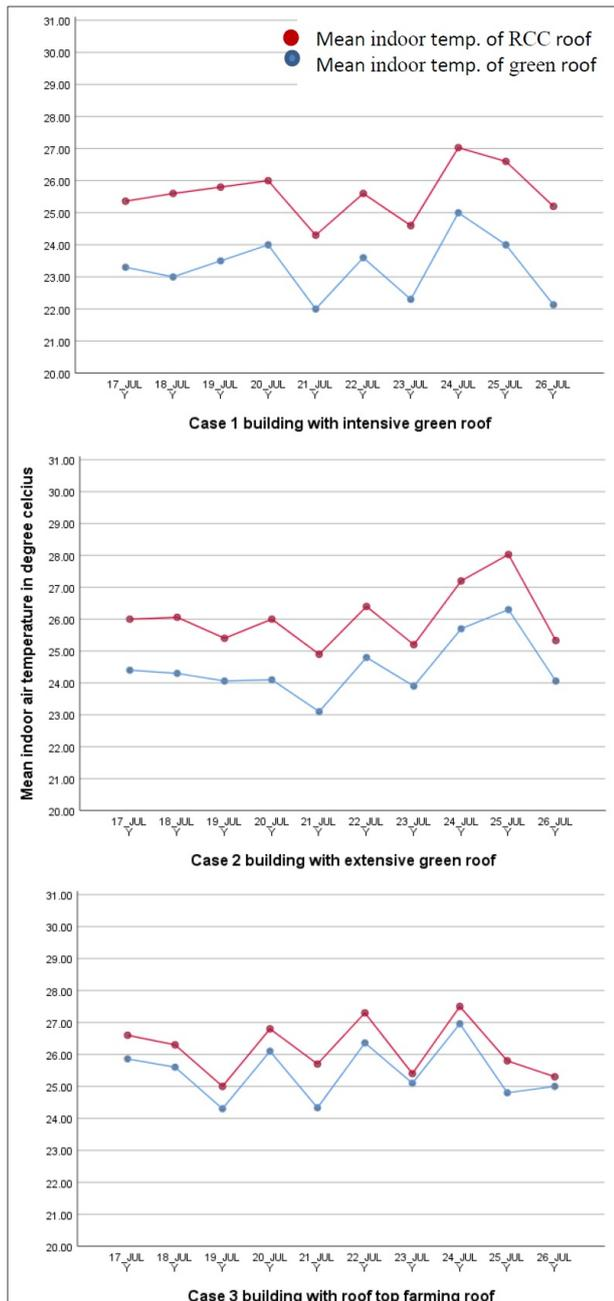
Figure 7: Comparison of mean indoor air temperature of green roof with RCC roof.
