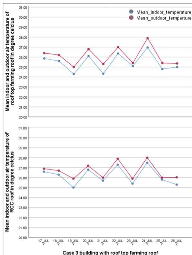
**Figure 11:** Comparison of mean indoor and mean outdoor air temperature of case 3 building.
