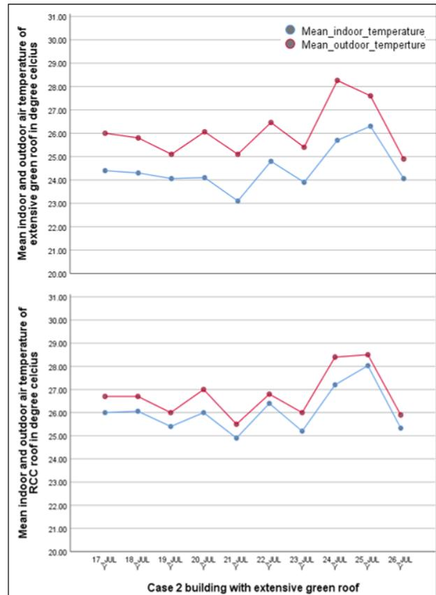
**Figure 10:** Comparison of mean indoor and mean outdoor air temperature of case 2 building.
