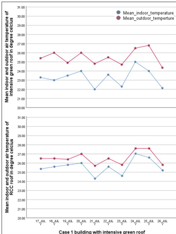
**Figure 9:** Comparison of mean indoor and mean outdoor air temperature of case 1 building.
