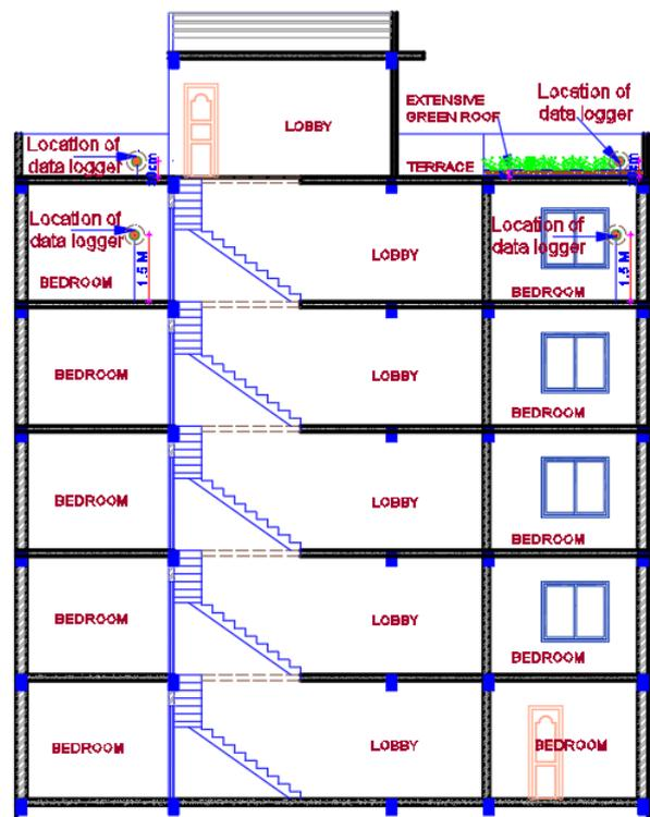
Figure 4: Building section of case 2 building with locations of data logger in indoor and outdoor of building for air temperature measurement.
