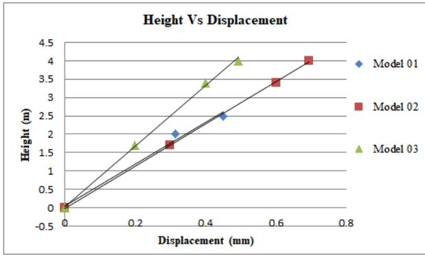
**Figure 4:** Height vs Displacement curve for different Models
