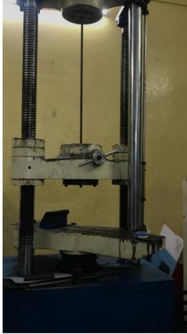
**Figure 2:** Setup for static load test
