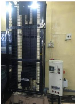
**Figure 3:** Setup for Relaxation test
