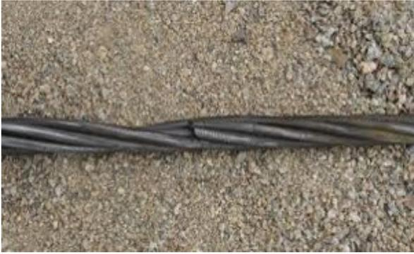
**Figure 19:** Breakage of Cable
