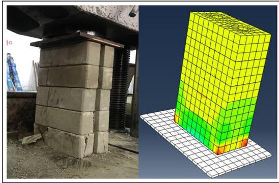
**Figure 3:** Failure of Masonry Prism (Experimental and Numerical Visualization)
