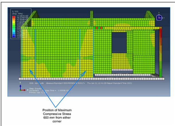
Figure 11: Stress around solid wall corners
