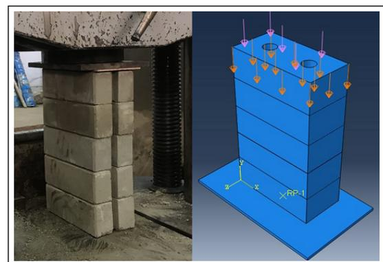
**Figure 2:** Physical Laboratory Setup and Numerical Model in Abaqus/CAE 2020
