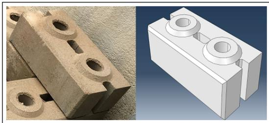
**Figure 1:** Typical CSEB interlock block used in analysis with its Solid Model
