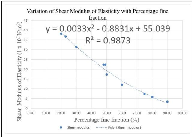
**Figure 2:** Variation of Shear Modulus of Elasticity with Percentage Fine Fraction in an Alluvial Deposits.
