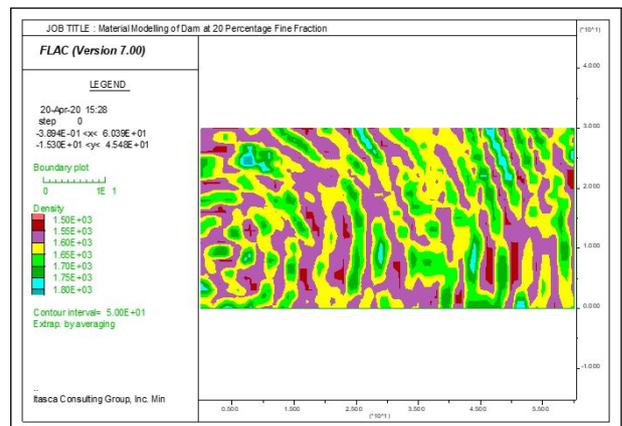
**Figure 13:** Density of Foundation Material at 20 percentage Fine Fraction.
