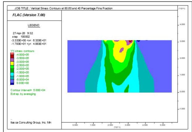
Figure 17: Vertical Stress Contours at layer of 80, 60 and 40 Percentage Fine Fraction.
