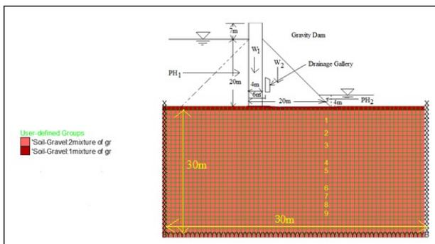
**Figure 28:** Modeling of Gravity dam at 35 Percentage fine fraction considering random heterogeneous distribution
