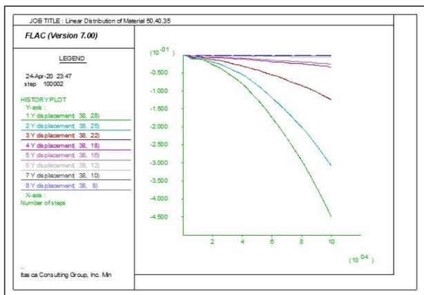
**Figure 21:** Vertical displacement histories at 8 different points.
