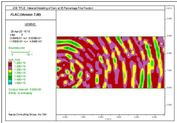
**Figure 9:** Bulk Modulus of Foundation Material at 35 percentage Fine Fraction.
