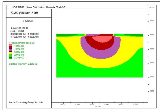
Figure 19: Vertical displacement contours at 50, 40 and 35 percentage fine fraction.
