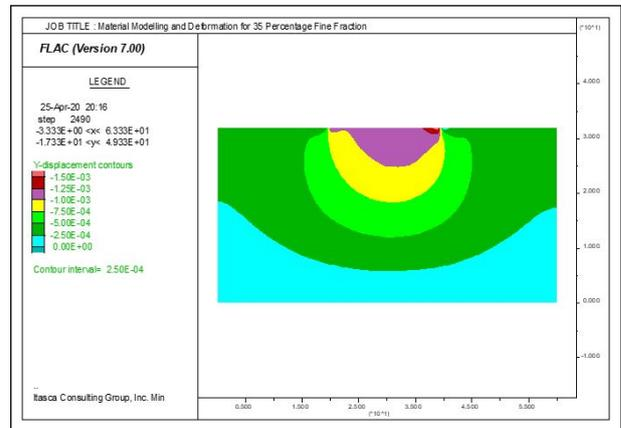
**Figure 30:** Vertical deformation of dam at 35 Percentage fine fraction considering random heterogeneous distribution.
