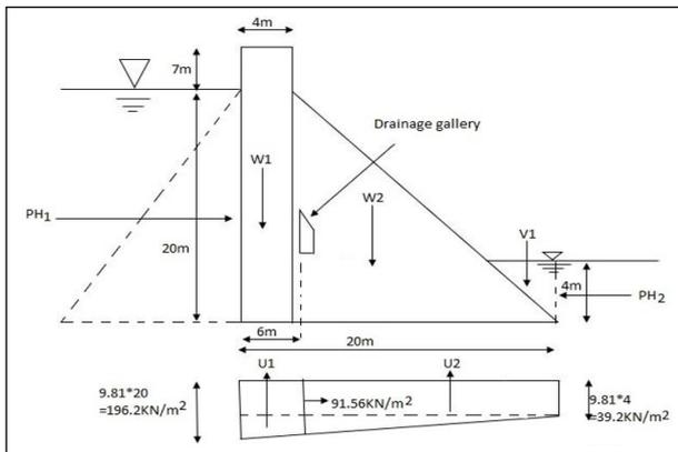
Figure 14: Gravity Dam.
