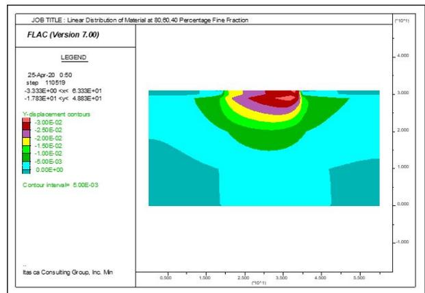
Figure 18: Displacement Contours of Dam at a layer of 80,60 and 40 Percentage Fine Fraction.
