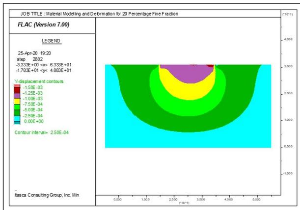
**Figure 33:** Vertical Displacement contours at 20 Percentage fine fractions considering random heterogeneous distribution.
