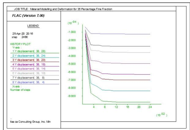
**Figure 31:** Vertical deformation histories of dam at 35 Percentage Fine fraction considering random heterogeneous distribution.
