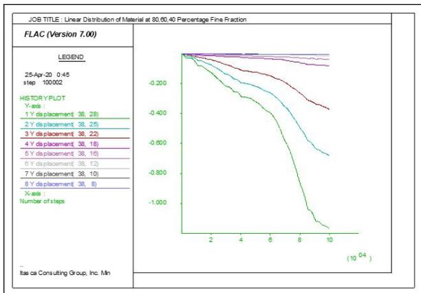
Figure 16: Deformation Histories of Dam at 8 different points.
