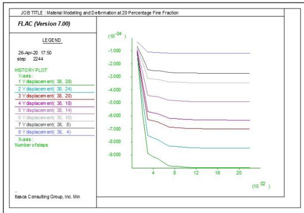
**Figure 32:** Deformation histories of dam at 8 different points considering random heterogeneous distribution.
