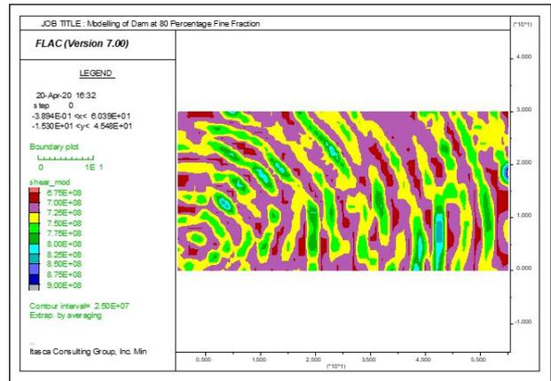
**Figure 5:** Shear Modulus of Foundation Material at 80 percentage Fine Fraction.
