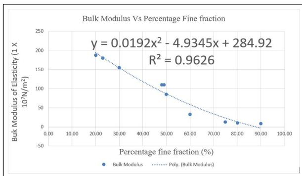
**Figure 4:** Variation of Bulk Modulus of Elasticity with Percentage Fine Fraction in an Alluvial Deposits.
