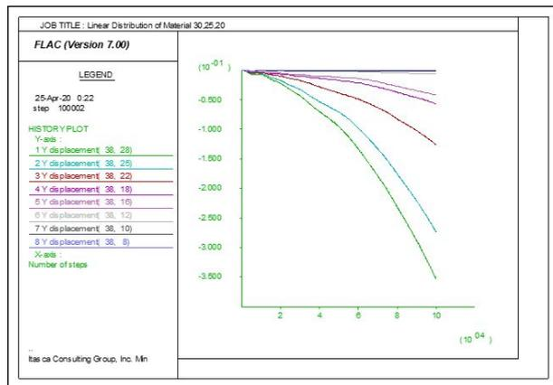
**Figure 23:** Vertical displacement Contours at 8 different points.
