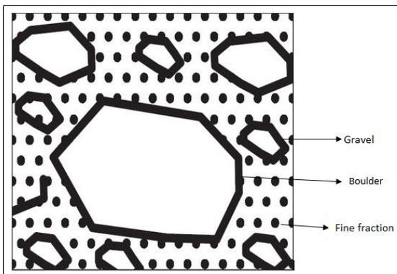
**Figure 1:** Alluvial mixture containing Boulder, Gravel and Fine fraction.
