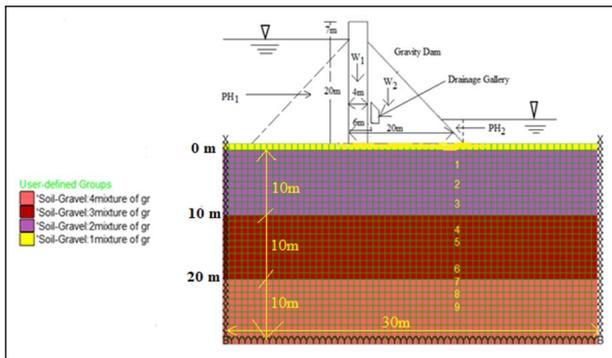
Figure 15: Model of Dam at layer of 80,60 and 40 Percentage Fine Fraction.
