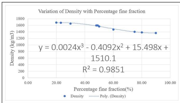
**Figure 3:** Variation of Density with Percentage Fine Fraction in an Alluvial Deposits.
