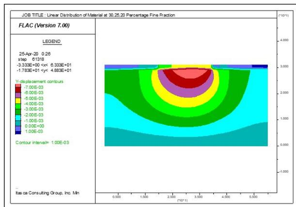
**Figure 24:** Vertical displacement contours at 30, 25 and 20 percentage fine fraction.
