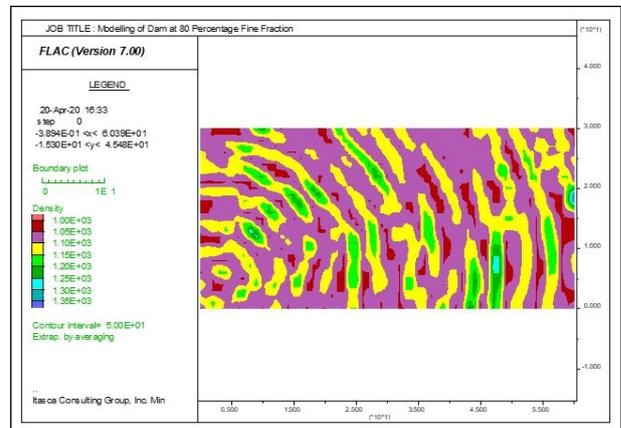
**Figure 7:** Density of Foundation Material at 80 percentage Fine Fraction.
