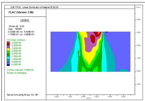
**Figure 22:** Vertical Stress Contours at 30, 25, and 20 Percentage Fine Fraction.
