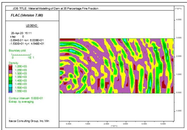
**Figure 10:** Density of Foundation Material at 35 percentage Fine Fraction.
