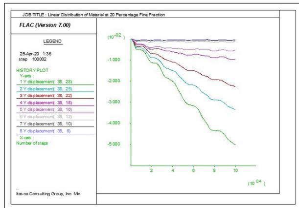
**Figure 25:** Displacement histories at 8 different points below toe of dam.
