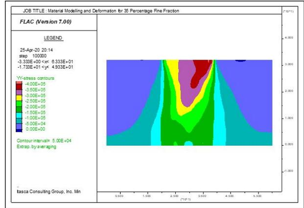
**Figure 29:** Vertical Stress Contours at 35 Percentage fine Fraction considering random heterogeneous distribution.
