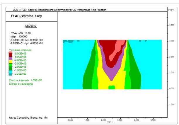
**Figure 34:** Vertical Stress contours at 20 Percentage fine fractions considering random heterogeneous distribution.
