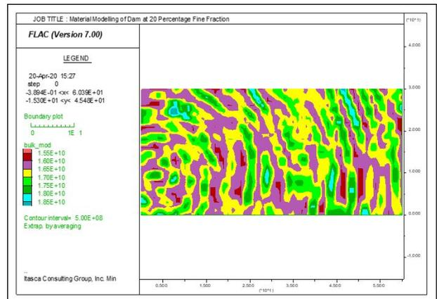
**Figure 12:** Bulk Modulus of Foundation Material at 20 percentage Fine Fraction.
