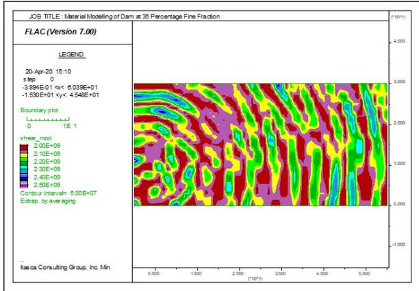
**Figure 8:** Shear Modulus of Foundation Material at 35 percentage Fine Fraction.
