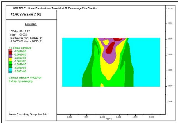
**Figure 27:** Vertical Stress Contours at 20 percentage fine fraction.
