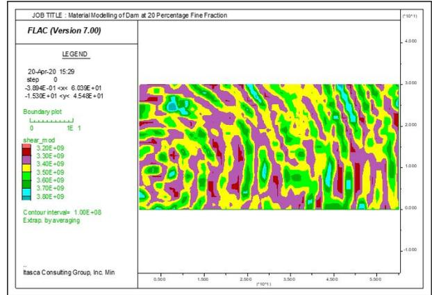
**Figure 11:** Shear Modulus of Foundation Material at 20 percentage Fine Fraction.
