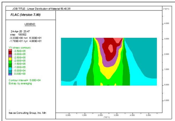
**Figure 20:** Vertical Stress contours at 50, 40 and 35 percentage fine fraction.
