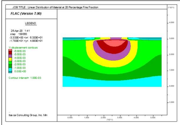
**Figure 26:** Vertical displacement of dam at 20 percentage fine fraction .
