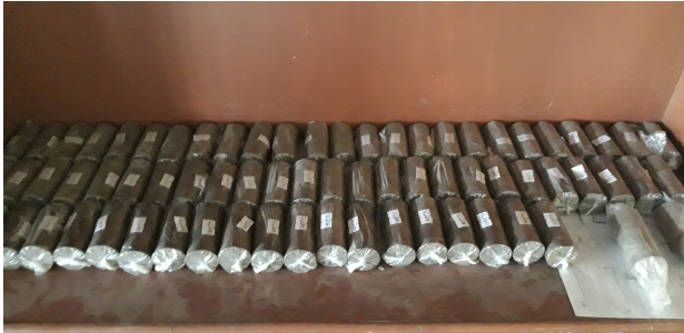
Figure 2: Samples kept for curing
