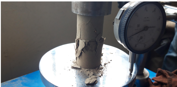
Figure 3: A Sample after UCS test
