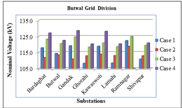
Figure 5: Voltage profile of Butwal grid substation
