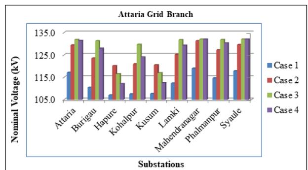
Figure 7: Voltage profile of Attaria grid substation
