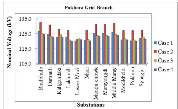
Figure 6: Voltage profile of Pokhara grid substation
