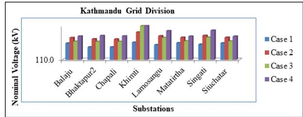
**Figure 1:** Voltage profile of Kathmandu grid substation
