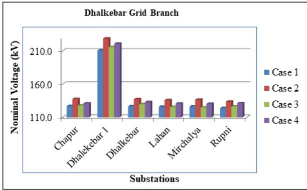
Figure 3: Voltage profile of Dhalkebar grid substation
