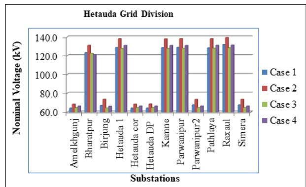
**Figure 2:** Voltage profile of Hetauda grid substation
