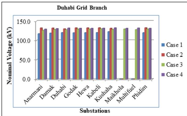
Figure 4: Voltage profile of Duhabi grid substation
