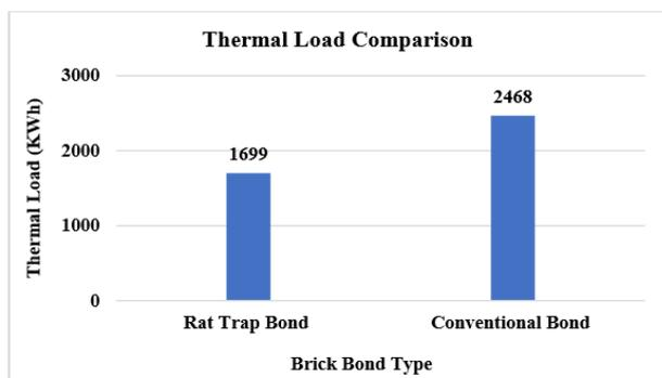
**Figure 2:** Thermal Load Comparison [7]
