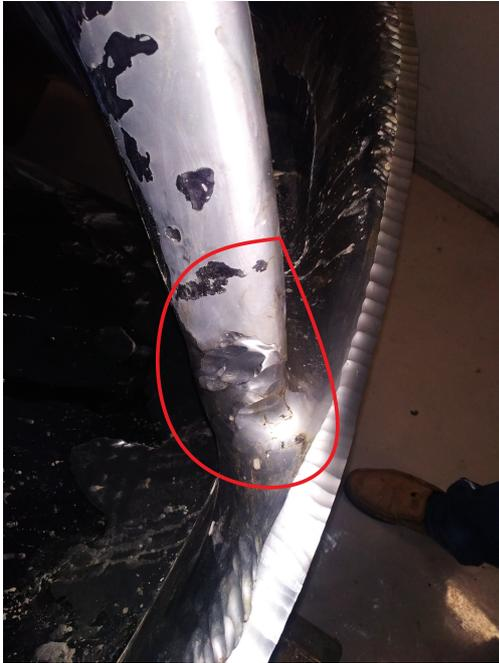
Figure 16: Erosion pattern in inlet side of the blade
