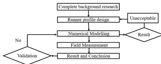
**Figure 1:** Different steps involved in case study of sand erosion in Francis turbine
