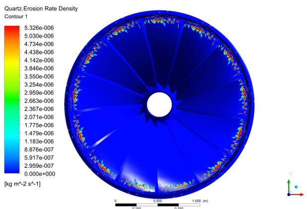
Figure 7: Erosion in runner outlet
