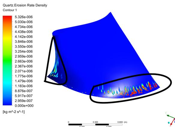
**Figure 15:** Erosion pattern in the runner blade via simulation
