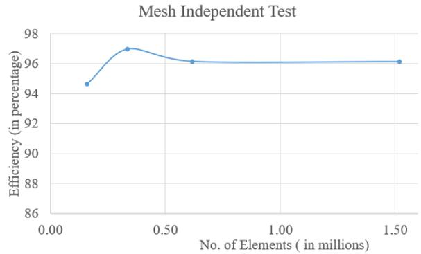
**Figure 5:** Mesh independence test for blade profile
