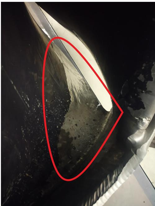
Figure 17: Erosion pattern in outlet side of the blade
