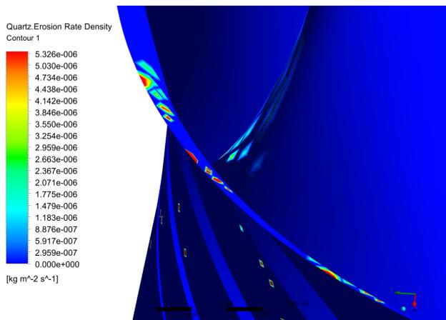
Figure 8: Erosion pattern in inlet side of runner
