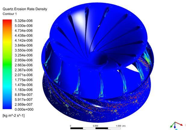
Figure 6: Erosion in runner
