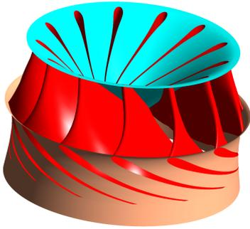
**Figure 3:** Runner profile of MMHPS designed in Bladegen
