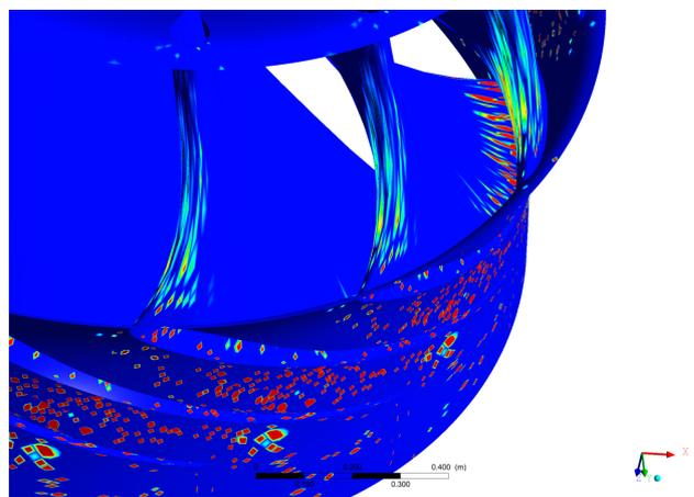
Figure 10: Erosion pattern in blade surface and outlet of runner
