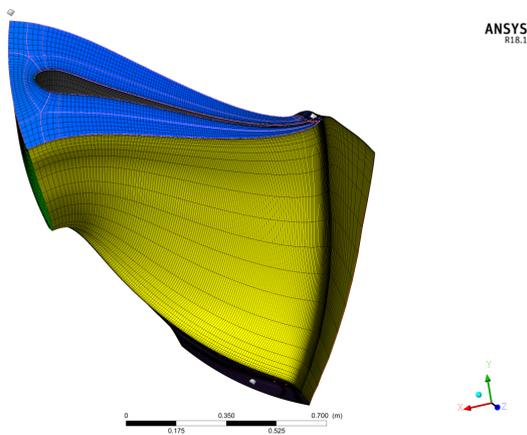
**Figure 4:** Mesh generation of blade domain in Turbo grid
