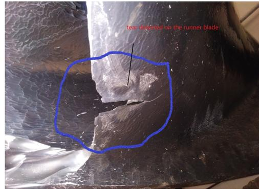
**Figure 13:** Tear detection at the outlet portion
