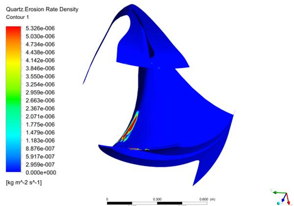
Figure 9: Erosion pattern in inlet side of blade
