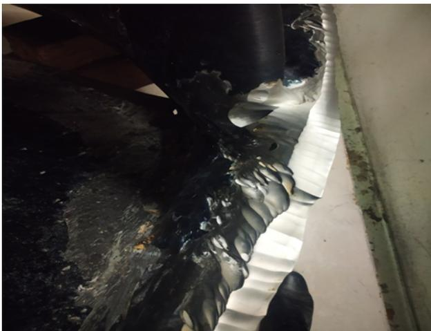
**Figure 12:** erosion on the inlet side of the runner
