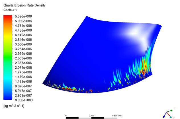
Figure 11: Erosion pattern in outlet side of blade
