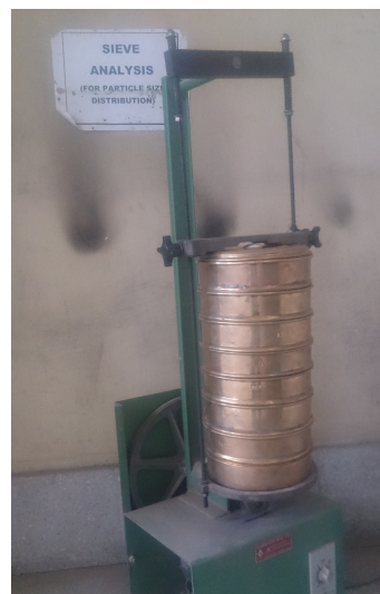
Figure 2: Arrangement for Sieve Analysis of Sawdust
