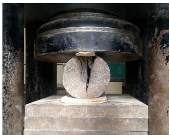
Figure 5: Cylinder Specimen at Failure Load
