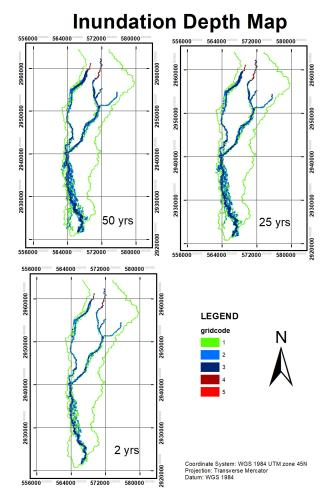
**Figure 4:** Inundation depth map of various return period
