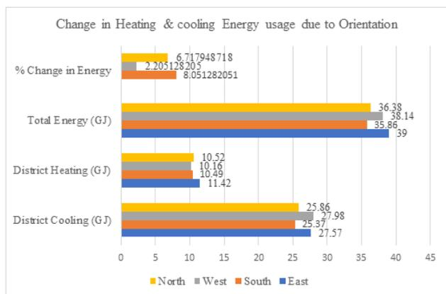
**Figure 35:** Change in heating and cooling energy usage due to orientation (LP Apartment)
