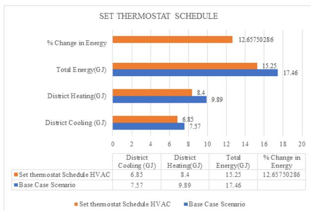
**Figure 24:** Comparison of result by setting thermostat schedule of HVAC (Guna Colony)
