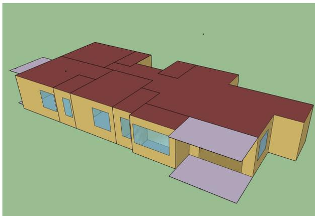
**Figure 19:** Energy model of LP Apartment in Sketchup- Openstudio with Energyplus
