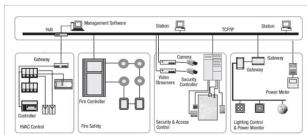
**Figure 6: Integrated Building System [11]**
