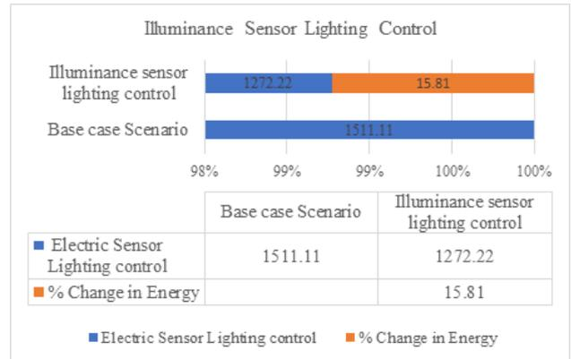
**Figure 31:** Comparison of electric lighting load by use of illuminance sensor lighting control (LP Apartment)
