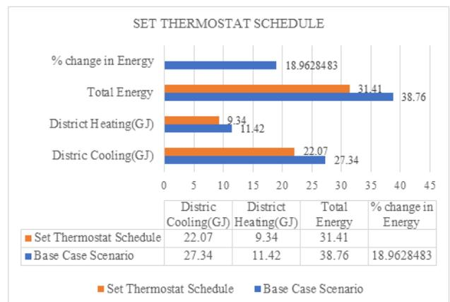
**Figure 33:** Comparison of result by setting thermostat schedule of HVAC (LP Apartment)
