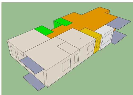
**Figure 21:** Energy model of LP Apartment render in terms of Thermal Zone
