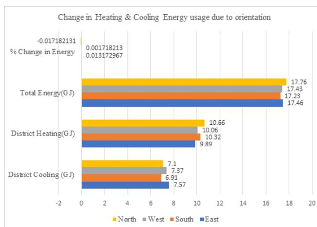
**Figure 26:** Change in heating and cooling energy usage due to orientation (Guna Colony)
