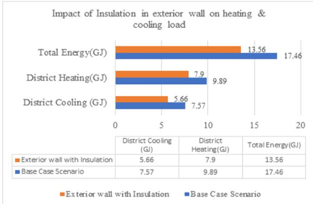
**Figure 28:** Impact of insulation in exterior wall on heating and cooling load (Guna Colony)
