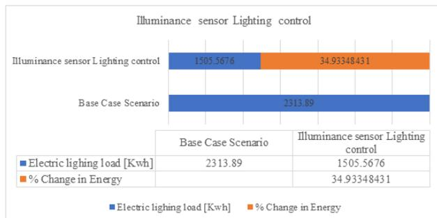
**Figure 22:** Comparison of electric lighting load by use of illuminance sensor lighting control (Guna Colony)
