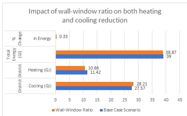
**Figure 36:** Impact of WWR on both heating and cooling reduction (LP Apartment)
