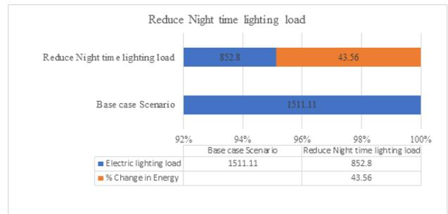
**Figure 32:** Comparison of electric lighting load by reduced night time lighting load (LP Apartment)
