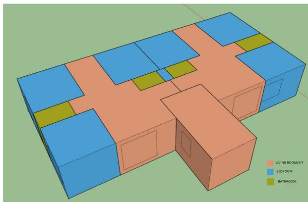
**Figure 17:** Energy model of Guna Colony Apartment render in terms of Space Type
