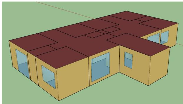
**Figure 16:** Energy model of Guna Colony Apartment in Sketchup- Openstudio with Energyplus
