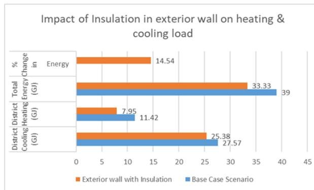
**Figure 37:** Impact of insulation in exterior wall on heating and cooling load (LP Apartment)
