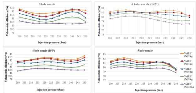
**Figure 6:** Interaction effect of injection pressure and load on volumetric efficiency for nozzles of different holes
