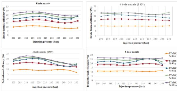
**Figure 4:** Interaction effect of injection pressure and load on brake thermal efficiency for nozzles of different holes
