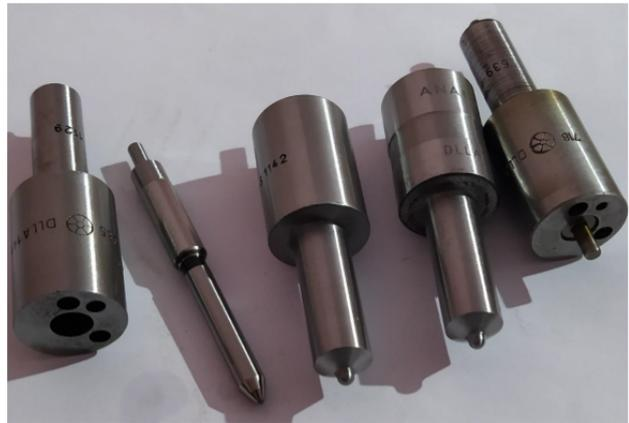
Figure 1: Fuel injector nozzles
