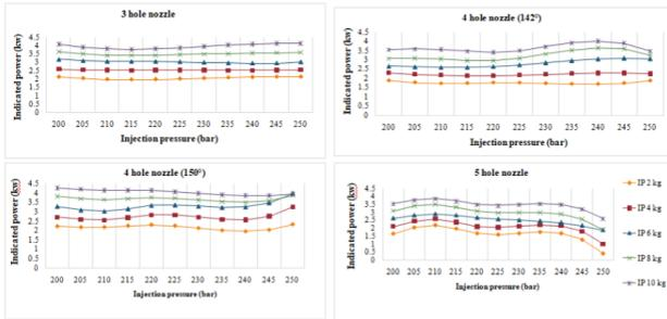
**Figure 3:** Interaction effect of injection pressure and load on indicated power for nozzles of different holes
