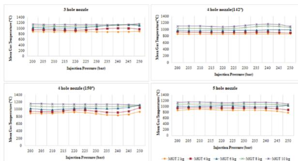
**Figure 10:** Interaction effect of injection pressure and load on mean gas temperature for nozzles of different holes
