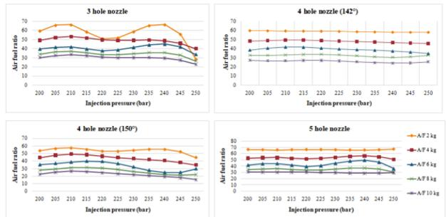
**Figure 7:** Interaction effect of injection pressure and load on air fuel ratio for nozzles of different holes
