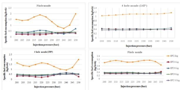
**Figure 5:** Interaction effect of injection pressure and load on specific fuel consumption for nozzles of different holes
