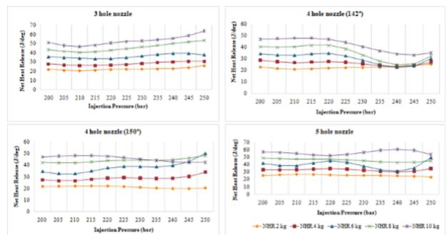
**Figure 8:** Interaction effect of injection pressure and load on net heat release for nozzles of different holes
